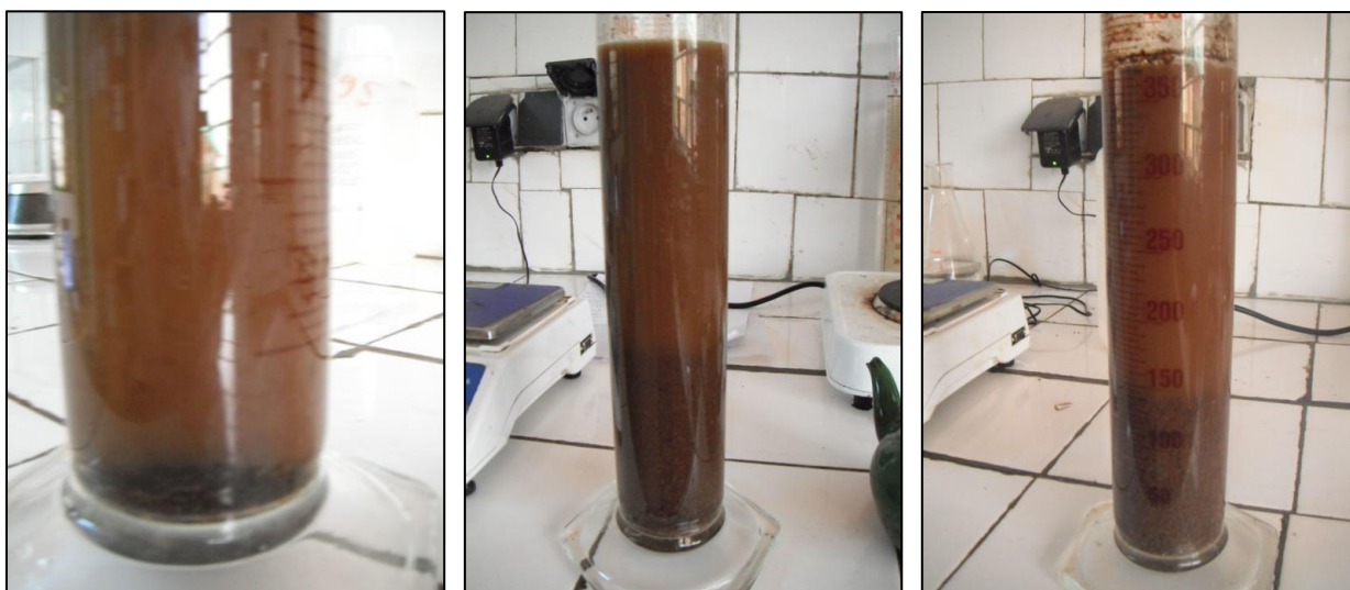
Figure 24: Sedimentation test; left : after a couple of minutes; middle : after 1 hour; right : after 3 days
